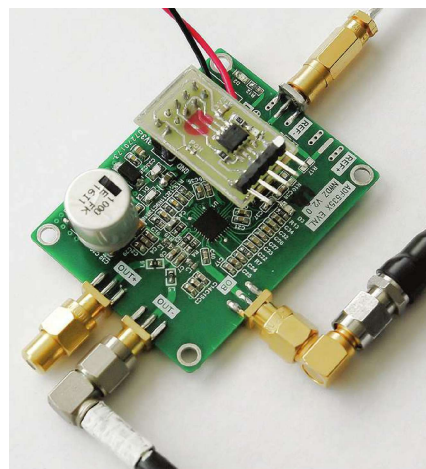
PHOTO 1: ADF5355 Fractional Synthesiser module from an eBay supplier. The small extra PCB carries a PIC for translating serial commands from a PC. The 1000 \mu F capacitor gives some extra supply decoupling to improve phase noise.
