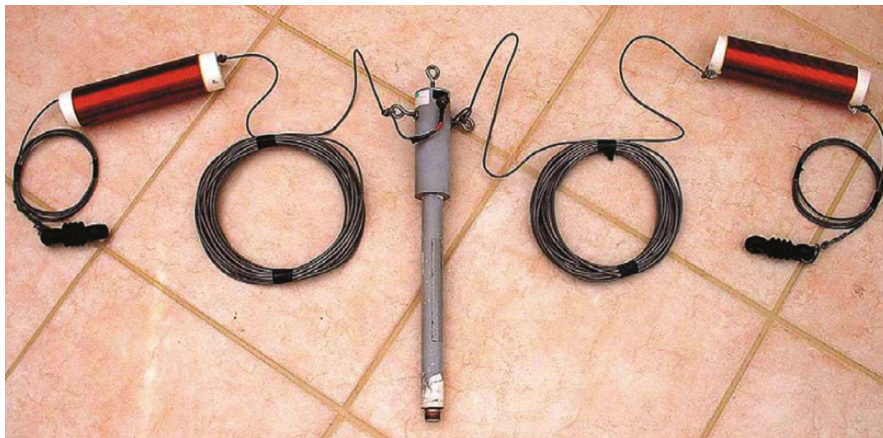
PHOTO 2: G3TKN's 80m & 40m loaded dipole that used a ferromagnetic 1:1 balun.
