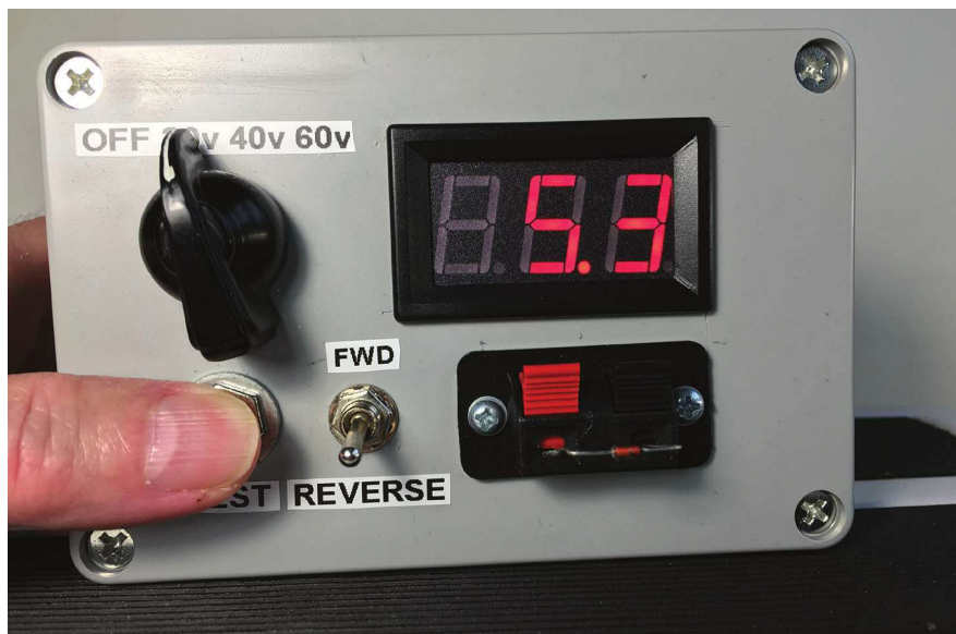
PHOTO 4: Testing a 5.3V Zener diode.
